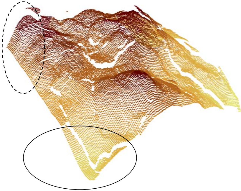
Fig. 4. Aggregate model. Dashed oval shows area of augmented probability. Solid lined oval shows area with reduced probability
